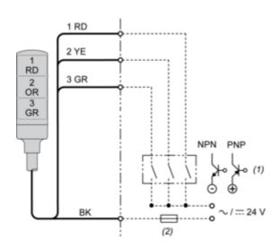
(1) "ON" for lighting and/or applying continuous sound.(2) Fuse (rated current: 0.5 A)
